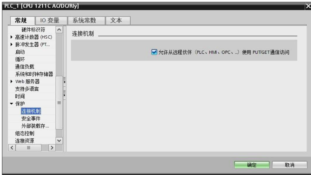
Figure 5-2-2 Enable remote access permission
